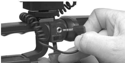
Figure 7 - Connecting the VideoMic lead to your camera
