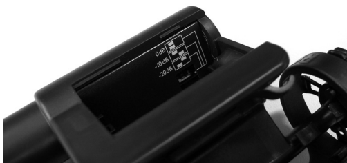
Figure 9 - Locating the PAD Switch
