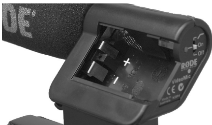
Figure 2 - The battery compartment
